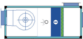
Supply Fan + Dry Steam Humidifier + Coil + Plate Filter + Mixing Box
