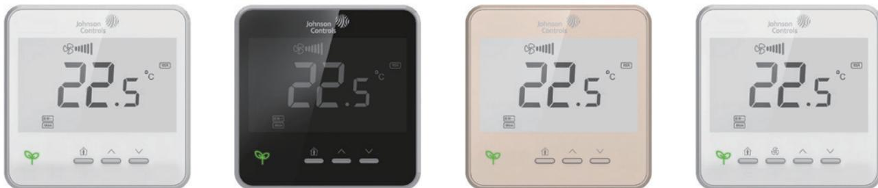
The flush-mounted NSA7000 series network sensor with LCD is an electronic zone sensor designed to function directly with Johnson Controls® BACnet® MS/TP digital controllers in heating, ventilating and air conditioning (HVAC) systems. Models in this series monitor the temperature set point, zone temperature and humidity, and transmit this data to a field controller on the sensor actuator (SA) bus.
