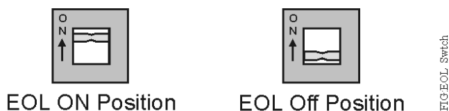
Figure 10: EOL switch positions
